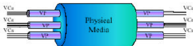
Figure 1: Relations between virtual path, virtual circuit and physical link
