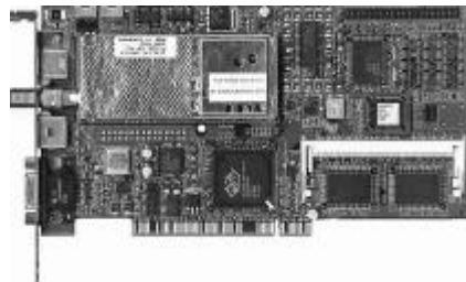
(PCI card - connectors also on other side, some pins not used by this card)
