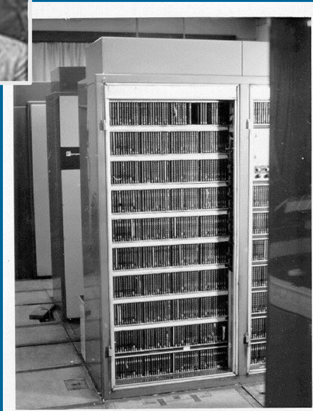
Atlas accumulator cabinet
