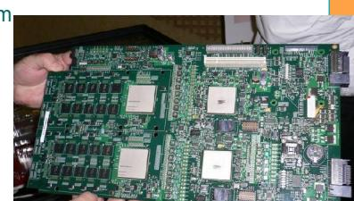
IBM Blade Server prototype w/ 2 cells (2005)
