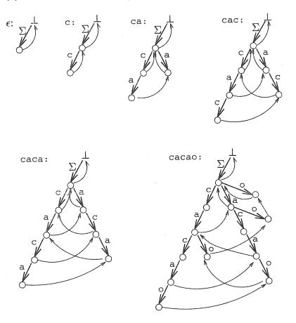
**Fig. 1.** Construction of STrie(cacao): state transitions shown in bold arrows, failure transitions in thin arrows. *Note:* Only the last two layers of suffix links shown explicitly.
