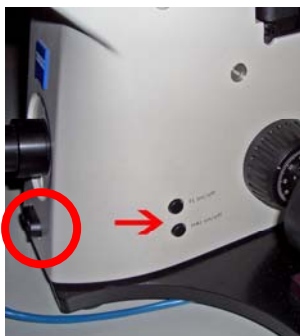
Figure 6. Red arrow: on/off button for transmitted light. Red circle: Transmitted light intensity adjustment.
