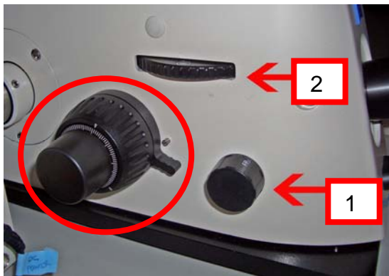
Figure 4. Adjustment of the light path to a correct port. Arrow 1: ocular/camera selection. Arrow 2: selection of the front/side port. Red circle: focusing knobs.
