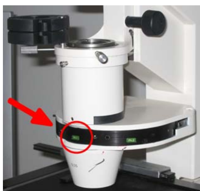
Figure 7. The position of the condenser.
