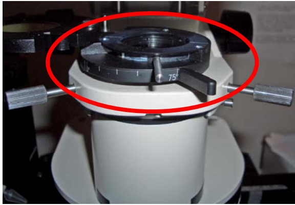
Figure 11 (left). The polarizer for DIC imaging. Figure 12 (right). The analyzer for DIC imaging.
