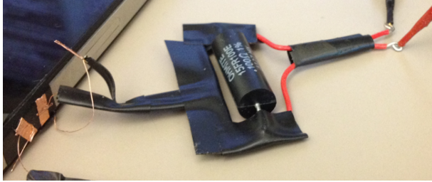
Figure 11. Close-up of the wiring rig that connects our iPhone 4S test phone with the Monsoon Power Monitor.
