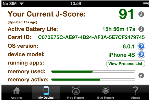
Figure 7. The Device tab on the iOS client. The J-Score indicates the percent of the community with worse battery life than this device.
