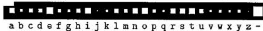
Figure 1.16. Probability distribution over the 27 outcomes for a randomly selected letter in an English language document (estimated from The frequently asked questions manual for Linux ). The picture shows the probabilities by the sizes of white squares.
