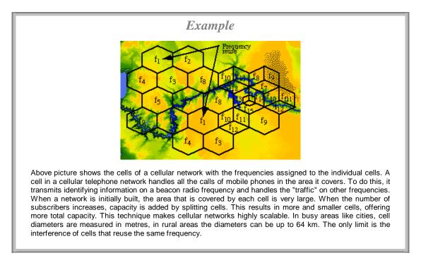
Figure 26: Example CellKeeper: picture showing a typical distribution of cells.
