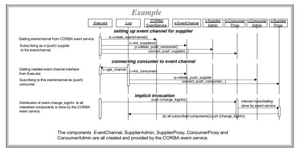
Figure 18: Example CellKeeper: mechanism for the implicit invocation of methods of the Log component
