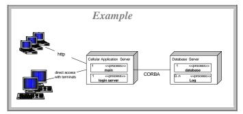
Figure 22: Example CellKeeper: hardware infrastructure
