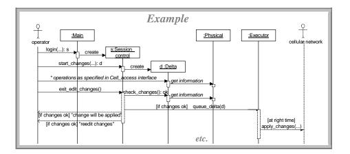
Figure 17: Example CellKeeper: an alternative component interaction model for the use case "OperatorChangingNetworkSession" specified in Figure 15
