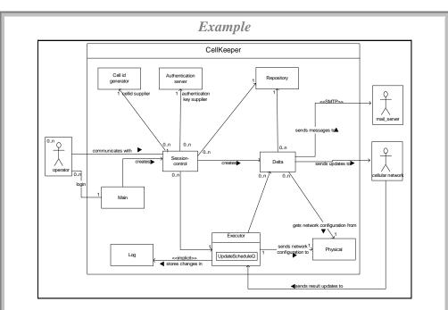
The CellKeeper system has one central repository for the cell management interfaces, one cell id generator, one authentication server and one executor. The system also contains an up-to-date model of the actual cellular network in the component physical. For each session with an operator, a Session\_control component is created. The component Log records all changes (failed and successful ones) that have been applied to the network.
