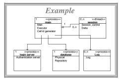
Figure 20: Example CellKeeper: static model of process view
