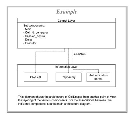
Figure 9: Example CellKeeper: Architecture diagram for the layering of the logical components
