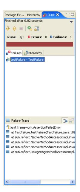
The view is shown in the current perspective whenever you start a test run. A convenient arrangement for the JUnit view is to dock it as a fast view. The JUnit view has two tabs: one shows you a list of failures and the other shows you the full test suite as a tree. You can navigate from a failure to the corresponding source by double clicking the corresponding line in the failure trace.
