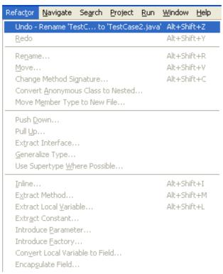
2. The refactoring changes are undone, and the workbench returns to its previous state. You can undo refactoring actions right up until you change and save a compilation unit, at which time the refactoring undo buffer is cleared.
