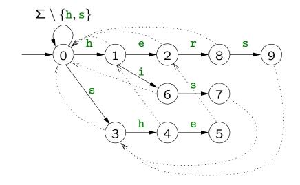
Algorithm 3.25: Aho-Corasick Input: text *T*, pattern set  $\mathcal{P} = \{P_1, P_2, \dots, P_k\}$ . Output: all pairs (i, j) such that  $P_i$  occurs in *T* ending at *j*. (1) Construct AC automaton (2)  $v \leftarrow root$ (3) for  $j \leftarrow 0$  to n - 1 do (4) while  $child(v, T[j]) = \bot$  do  $v \leftarrow fail(v)$ (5)  $v \leftarrow child(v, T[j])$ (6) for  $i \in patterns(v)$  do output (i, j)
