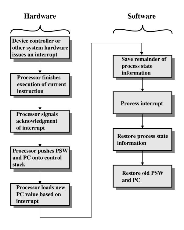
**Figure 1.10 Simple Interrupt Processing**
