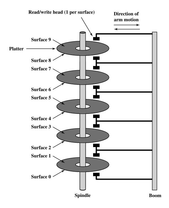
Figure 11.18 Components of a Disk Drive
