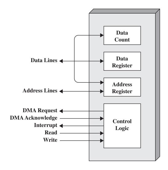
Figure 11.2 Typical DMA Block Diagram
