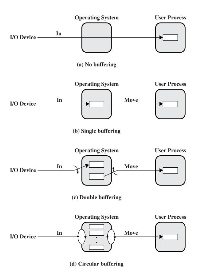
Figure 11.6 I/O Buffering Schemes (input)
