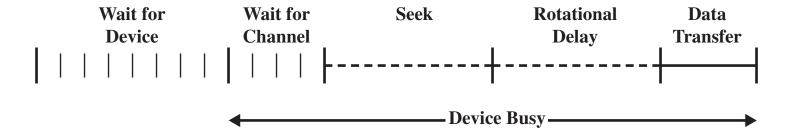
Figure 11.7 Timing of a Disk I/O Transfer
