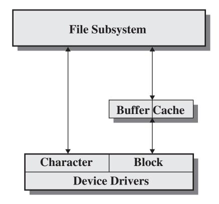
Figure 11.14 UNIX I/O Structure
