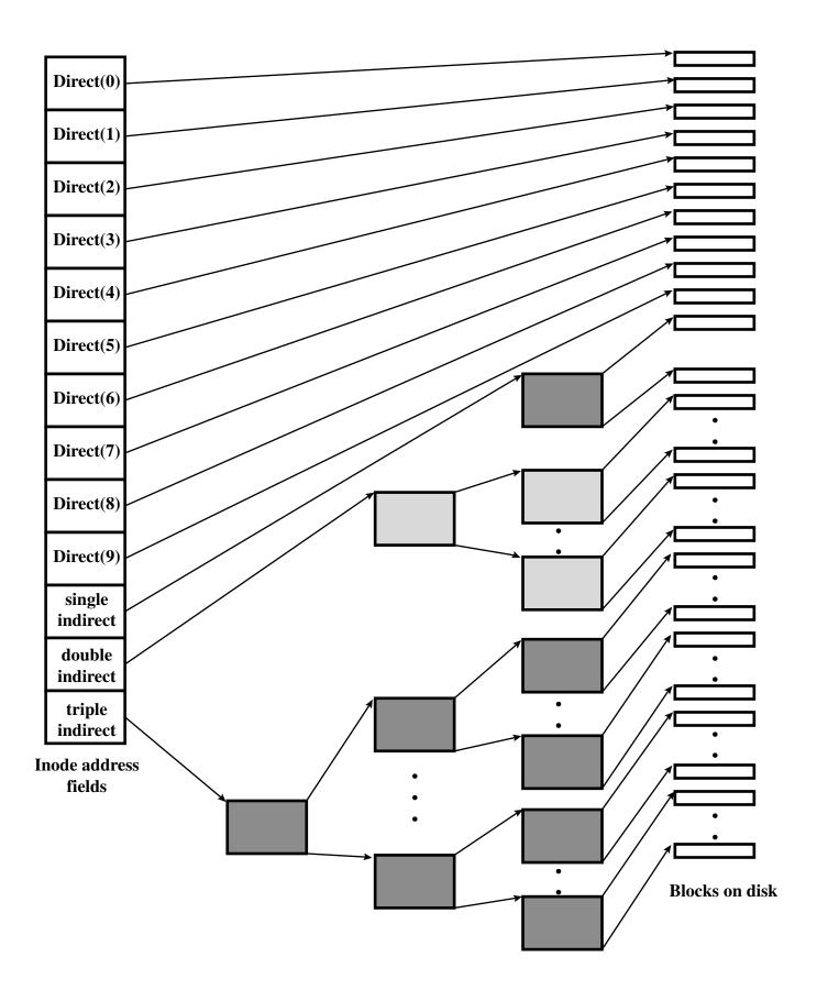
Figure 12.13 UNIX Block Addressing Scheme
