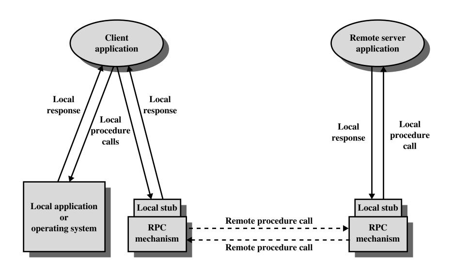
**Figure 13.13 Remote Procedure Call Mechanism**
