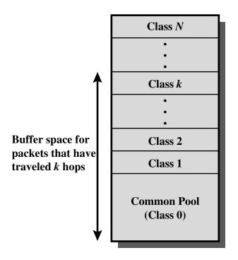
**Figure 14.18 Structured Buffer Pool for Deadlock Prevention**
