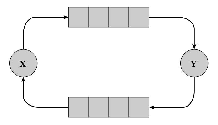
Figure 14.19 Communication Deadlock in a Distributed System
