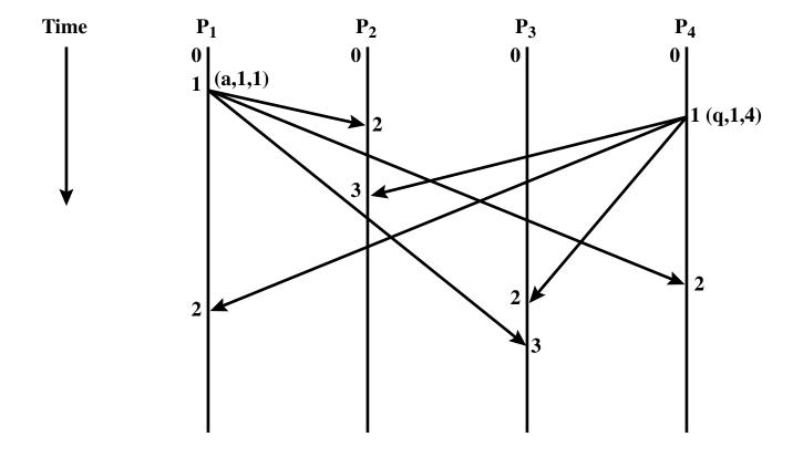
Figure 14.9 Another Example of Operation of Timestamping Algorithm
