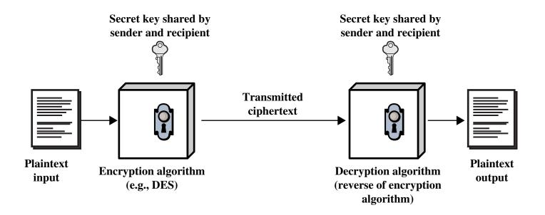
Figure 15.13 Simplified Model of Conventional Encryption
