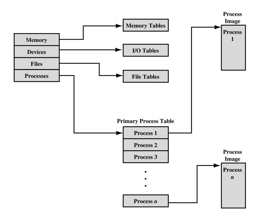
Figure 3.10 General Structure of Operating System Control Tables
