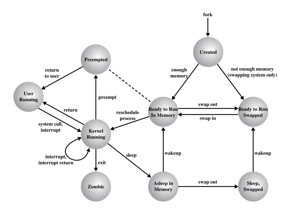
**Figure 3.16 UNIX Process State Transition Diagram**
