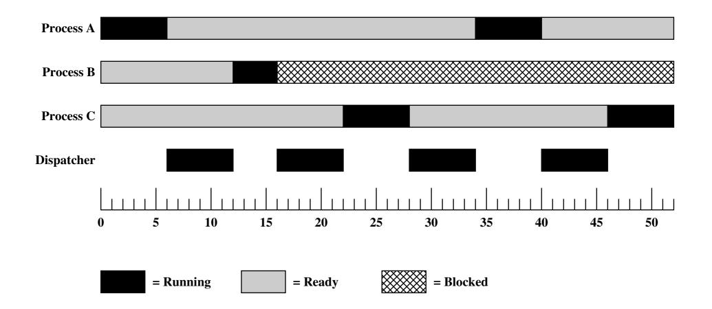
Figure 3.6 Process States for Trace of Figure 3.3
