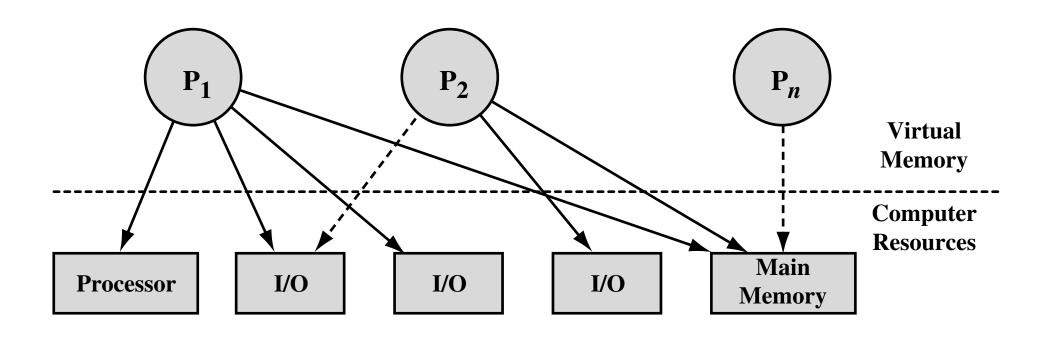
Figure 3.9 Processes and Resources (resource allocation at one snapshot in time)
