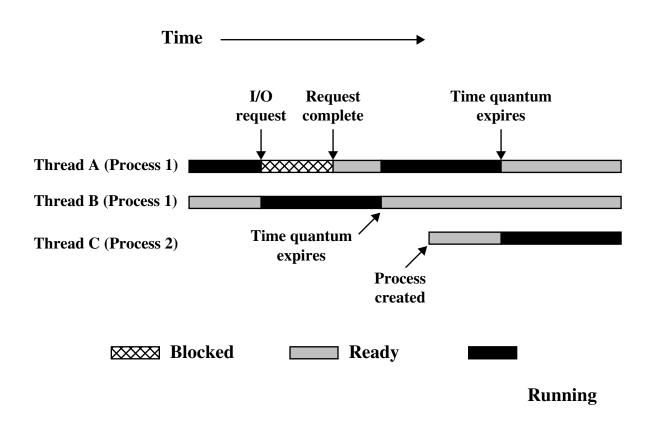
Figure 4.4 Multithreading Example on a Uniprocessor
