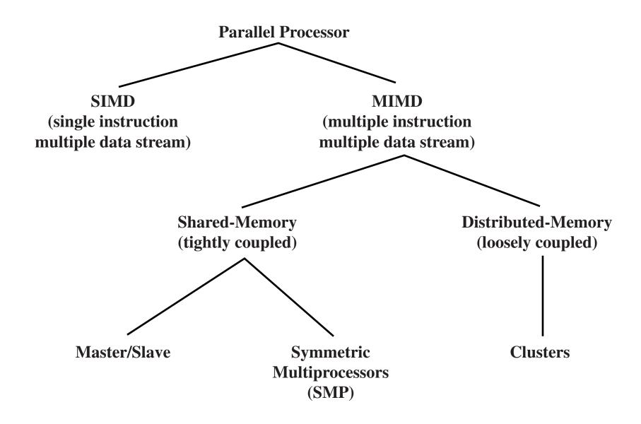
Figure 4.8 Parallel Processor Architectures
