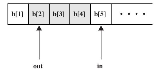
Note: shaded area indicates portion of buffer that is occupied
