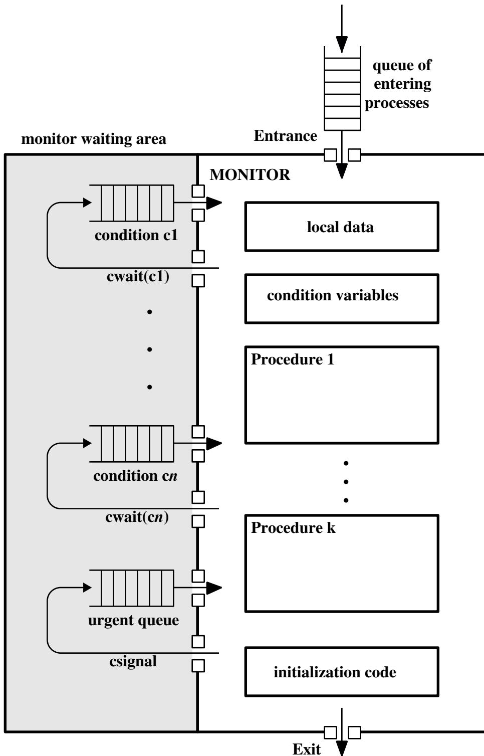
**Figure 5.21 Structure of a Monitor**
