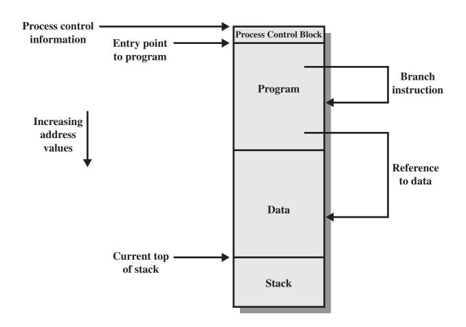
Figure 7.1 Addressing Requirements for a Process
