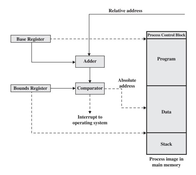
**Figure 7.8 Hardware Support for Relocation**
