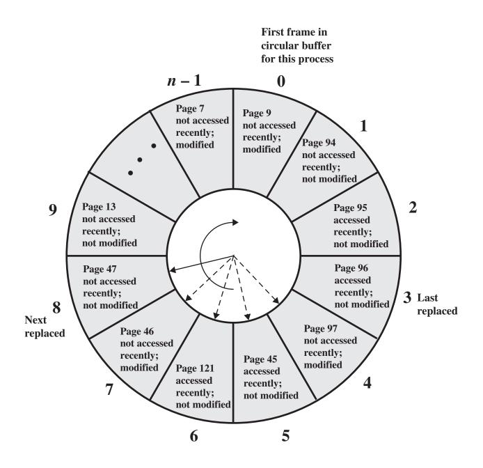
Figure 8.18 The Clock Page-Replacement Algorithm [GOLD89]
