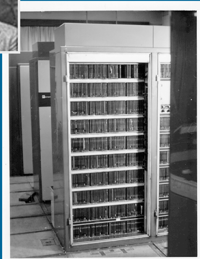
Atlas accumulator cabinet
