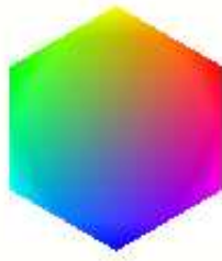
Figure 6: The colour hexagon used for analyzing the colour content of the PCA and ICA basis patches. The hexagon is the projection of the RGB cube onto a plane orthogonal to the luminance ( R + G + B ) vector. Thus achromatic RGB triplets map to the center of the hexagon while highly saturated ones are projected close to the edges.
