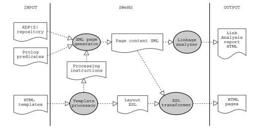
Figure 2: Internal architecture of SWeHG.
