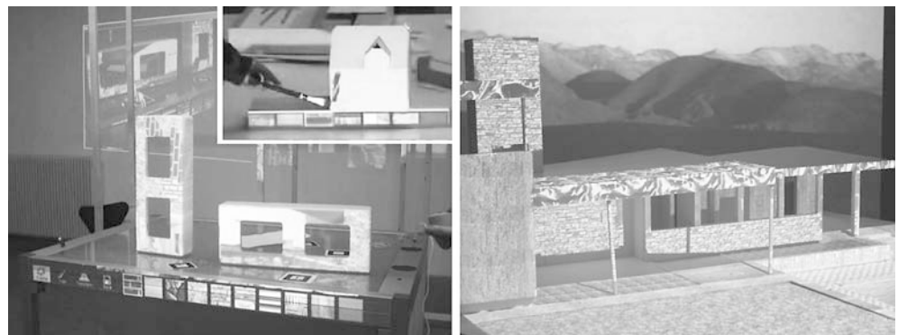
Fig. 9 Configuring the Texture Brush for painting a model ( left ), on the border of the table is the menu bar. A painted model from two directions with background ( right )
