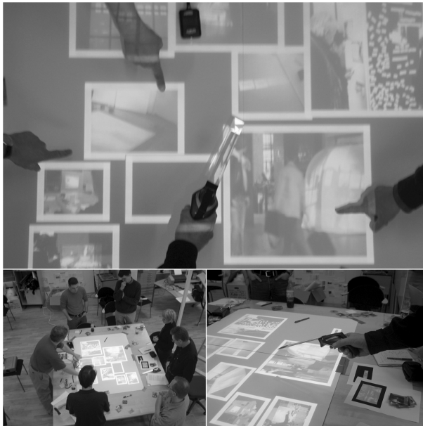
Fig. 7. The Tracking Game Table is a set-up which uses a tracking system, allowing manipulation of virtual frames in which images and videos are displayed. A specially designed wireless mouse communicates with the tracking system by a reflector. The frames can be moved around, scaled to different sizes and videos can be started and paused. Playing cards augmented with RFID tags carry links to media files, and when a selected card is held above a tag reader, the media is displayed in a new frame
