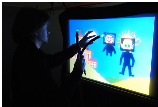
Figure 2. Prototype of PuppetWall and a user holding a MagicWand in their right hand and interacting with a prop with their left. There are two characters on the stage, partially hiding two props (then sun and a bicycle).
