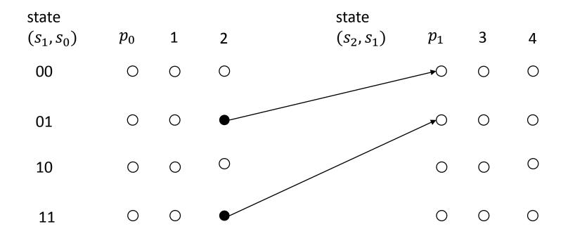
Also, there are such situations when two paths enter one node in that case path with minimal weight is chosen as a survivor. Similarly, all bits of partial syndrome are calculated, and in the end of the trellis the only one path with minimal weight is chosen.
