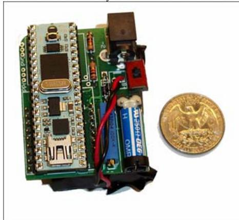
Fig. 8. Custom telemetry device, which consists of accelerometer, microcontroller, and transmitter. Battery is attached to the rear side of the board. Dimensions are 5.1 cm x 4.2 cm x 2.0 cm.
