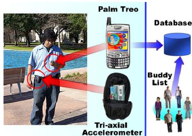
Fig. 7. Player wears activity sensor at his waist and holds a Palm Treo PDA phone at his palm. The devices are indexed in the right panel where the connectivity architecture is also shown.
