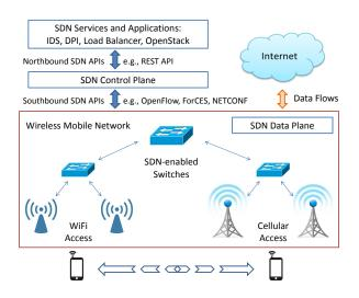
Fig. 1: SDN-enabled Wireless Mobile Networks
