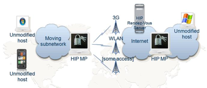
In the current Internet architecture hosts are identified and located by IP addresses Instead of IP addresses, HIP uses a new cryptographic namespace for identification
