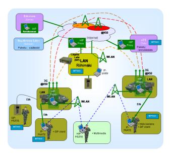
HIP protocol suite is standardized in the IETF Ericsson Finland is one of the main drivers Prototypes exist for the whole protocol suite Mobile Proxy allows use of legacy end hosts
