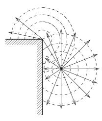
Figure 2.3: Diffraction.
