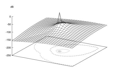
Figure 4.2: An illustration of the average attenuation evaluated using Equation (4.2). The transmitter is located in the center of the area and its direction of transmission is towards the upper right corner of the area.
