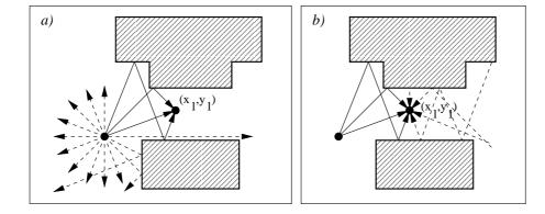
Figure 2.5: Ray-optical models: (a) ray-launching, and (b) ray-tracing. The rays which affect the field at point  $(x_1, y_1)$  are denoted by solid arrows. The transmitter is denoted by the black dot on the left side of the obstruction.
