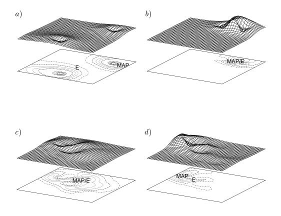
Figure 4.6: Examples of the posterior p.d.f. of the location variable with different signal strength observations. Labels indicate the maximum a posteriori estimate ("MAP"), and the expected value ("E") of the location variable. In graphs (b) and (c) they are practically identical.
