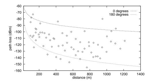
Figure 4.3: Mean path loss curves obtained from sample data. Small blots represent observed path loss values at varying distances from the transmitter. The two curves show the mean path loss to the direction of transmission  $(\delta = 0^{\circ})$ , and to the opposite direction  $(\delta = 180^{\circ})$ .
