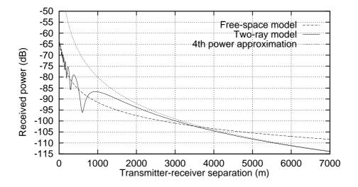
Figure 2.2: The received power referenced to the transmitted power as a function of the transmitter-receiver distance according to the free-space model (Equation (2.7)), the two-ray model (Rappaport, 1996, p. 87), and the fourth-power approximation of the two-ray model (Equation (2.8)). The parameters are: transmitter elevation = 50 m, receiver elevation = 2 m, frequency = 900 MHz, relative permittivity of the ground = 15, antenna gains and system loss = 1.0 (no loss).
