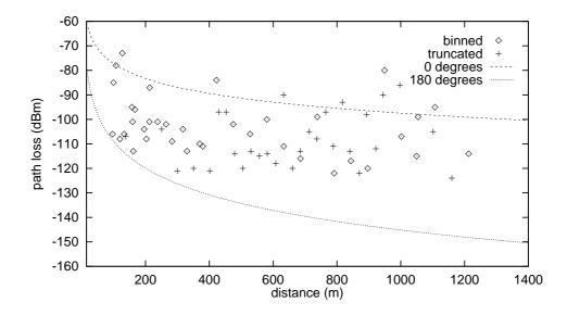
Figure 4.4: Mean path loss curves obtained from sample data. Small symbols represent binned ( $\diamond$ ) and truncated (+) path loss values at varying distances from the transmitter. The two curves show the mean path loss to the direction of transmission ( $\delta = 0^{\circ}$ ), and to the opposite direction ( $\delta = 180^{\circ}$ ).
