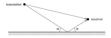
Figure 2.1: Two-ray ground reflection model.
