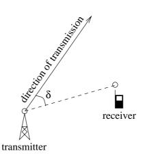
Figure 4.1: The deviation,  $\delta$ , between the direction of transmission and the direction of the receiver as measured from the transmitter.
