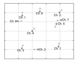
Figure 4.5: A hypothetical network layout consisting of ten transmitters. Arrows indicate direction of transmission, and labels indicate channels. Note that channels one and two are both shared by two transmitters.
