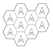
Figure 1.1: An idealized diagram of a cellular network layout.
