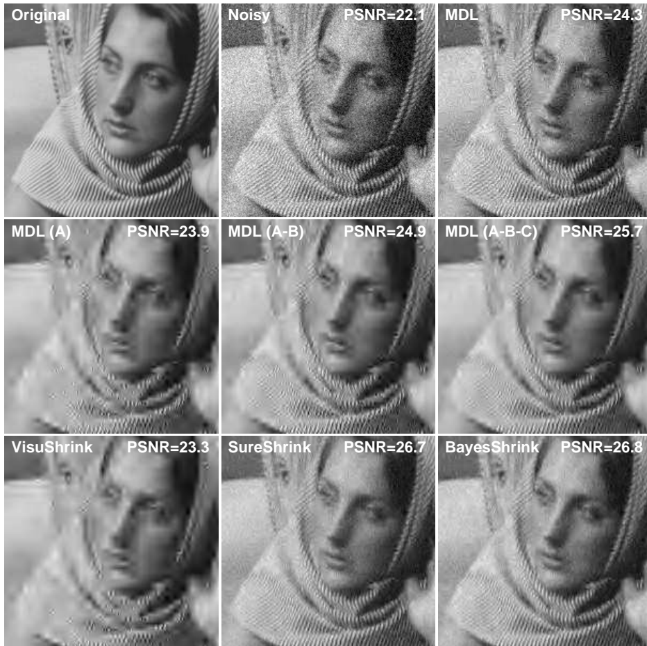
Figure 8.3: Barbara image (detail). First row : original image; noisy image, noise standard deviation \sigma = 20.0 ; original MDL method [105]. Second row : MDL with refinement A; MDL with refinements A and B; MDL with refinements A, B, and C. Third row : VisuShrink; SureShrink; BayesShrink. Peak-signal-to-noise ratio (PSNR) in decibels is given in each panel. (Higher PSNR is better).
