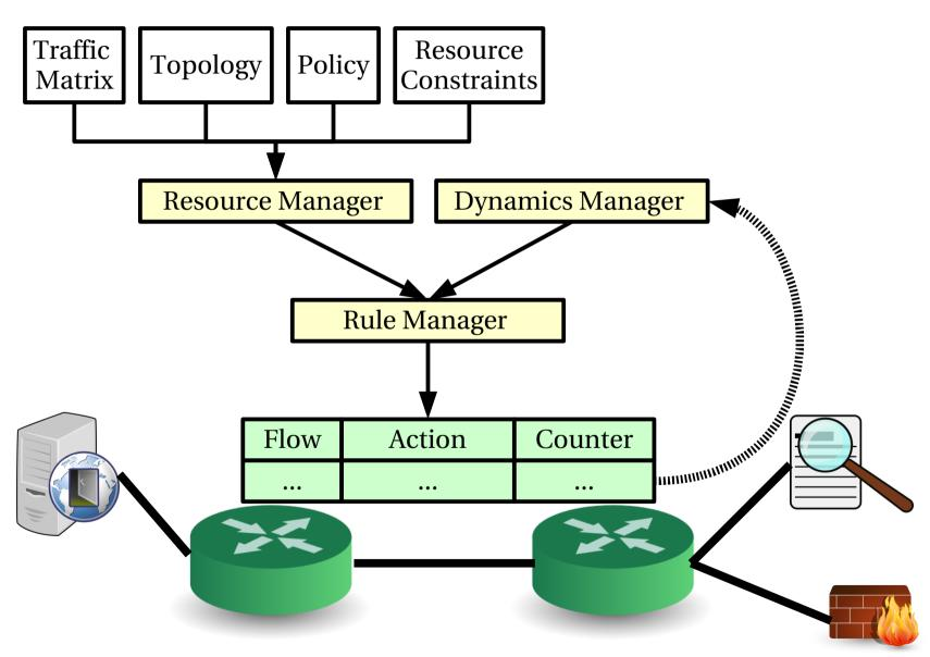
SDN based Policy Enforcement Layer for NFspecific traffic steering
