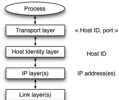
Fig. 1. Approximate location of the HIP sublayer within the TCP/IP stack.
