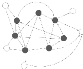
Figure 1. Graph defined by link structure of web pages. The dark nodes construct a strongly self-referring set with threshold min_f = 2/3 .
