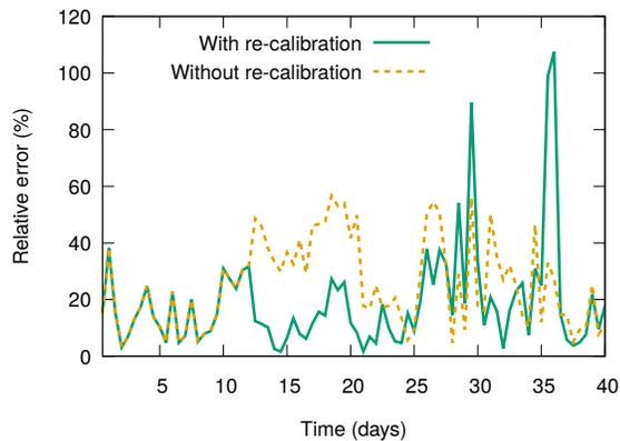
**Figure 2: Relative error of mini-SMEAR  $O_3$  measurements calibrated against SMEAR. *With re-calibration* is re-calibrated every 14 days.**
